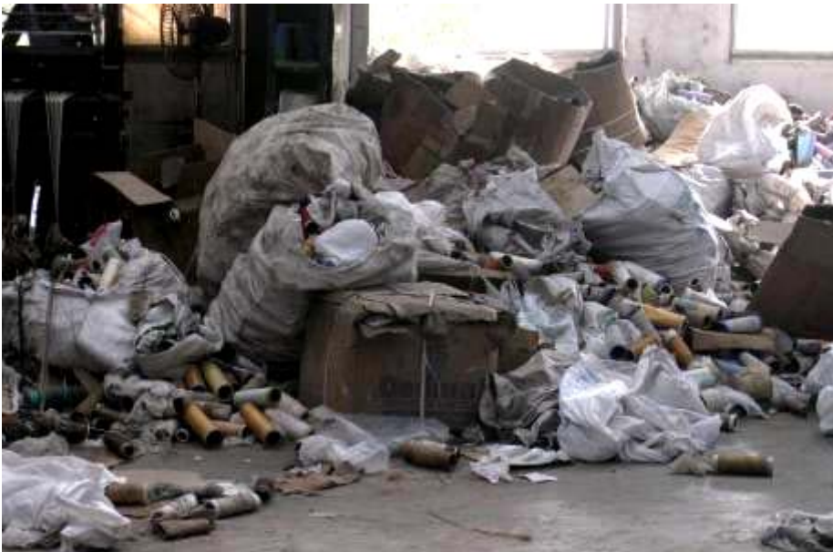
Flammable garbage in a plant
