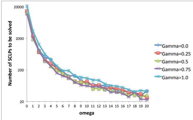
(b) Effect of  $\omega$  on reducing the number of times we solve Problem (11). Note that the  $y$ -axis is in a logarithmic scale.Fig. 3. Effect of  $\omega$ . Results for the criss-cross network of Figure 1 under the traffic case B.H. and different values of  $\Gamma$  and  $\Omega$ .
