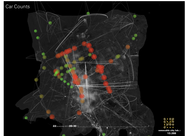
Figure 6: The extracted Origin Destination (OD) matrix across Riyadh at the time slice of 9:30-9:45am. The height of the line corresponds to the number of trips between a specific OD.
