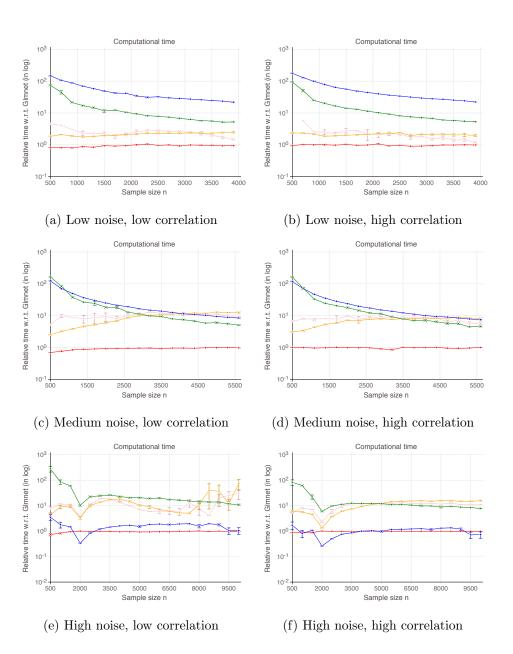
Fig 2: Computational time relative to Lasso with glmnet as n increases, for CIO (in green), SS (in blue with  $T_{max} = 200$ ), ENet (in red), MCP (in orange), SCAD (in pink) with OLS loss. We average results over 10 data sets.
