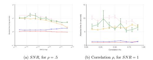
Fig 16: Absolute computational time as signal-to-noise or correlation increases, for CIO (in green), SS (in blue with  $T_{max} = 200$ ), ENet (in red), MCP (in orange), SCAD (in pink) with OLS loss. We fixed p = 5,000,  $k_{true} = 50$ , and n = 1,000, and averaged results over 10 data sets. We report results of CIO and SS with  $k = k_{true}$  and  $\gamma = \frac{p}{2n k_{true} \max_i ||x_i||^2}$ .
