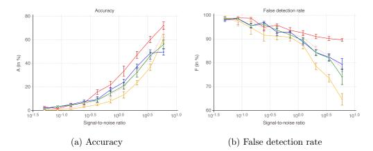
Fig 9: Accuracy and false detection as SNR increases, for the CIO (in green), SS (in blue with  $T_{max} = 150$ ), ENet (in red), MCP (in orange), SCAD (in pink) with OLS loss. We average results over 10 data sets with SNR = 0.05, ..., 6,  $k_{true} = 50$ .
