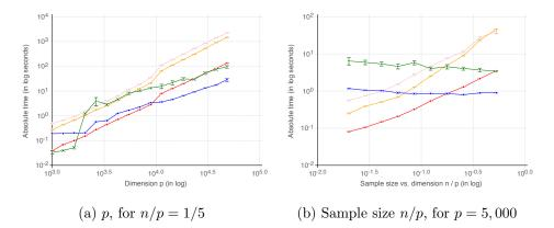
Fig 17: Absolute computational time as dimension p or sample size n increases, for CIO (in green), SS (in blue with  $T_{max} = 200$ ), ENet (in red), MCP (in orange), SCAD (in pink) with OLS loss. We fixed  $p = 5,000, k_{true} = 50$  and averaged results over 10 data sets. We report results of CIO and SS with  $k = k_{true}$  and  $\gamma = \frac{p}{2n k_{true} \max_i ||x_i||^2}$ .
