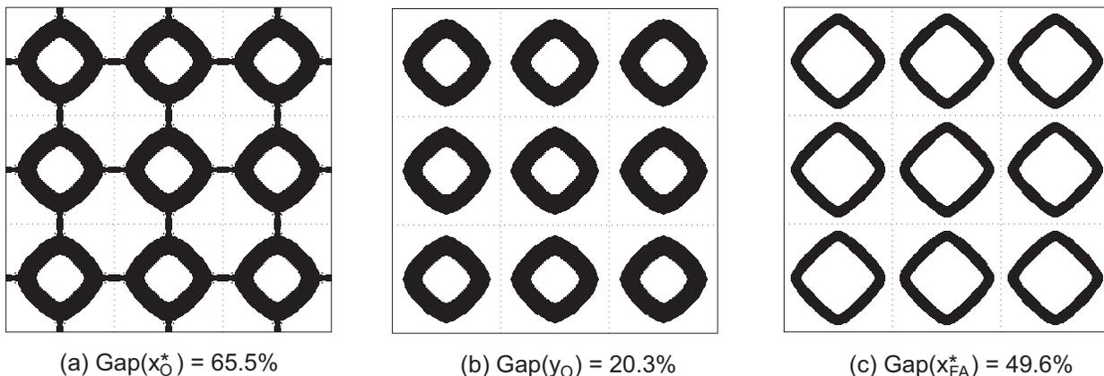
**Figure 3** Solutions to the 2nd TE bandgap problem in the square lattice. (a) is the original optimal design  $x_O^*$ , with  $\text{Gap}(x_O^*) = 65.5\%$ ; (b) is the solution  $y_O$  which is a manual modification of  $x_O^*$ , with  $\text{Gap}(y_O) = 20.3\%$ , and 3% of pixels being modified; (c) is the computed solution  $x_{FA}^*$  of using Algorithm FA-B, with  $\text{Gap}(x_{FA}^*) = 49.6\%$ , using  $\delta = 3\%$ .
