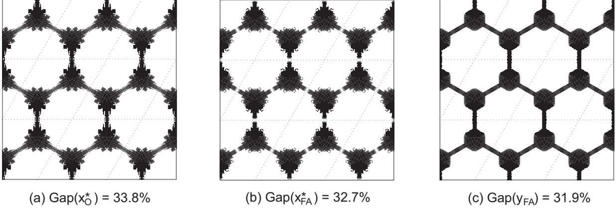
**Figure 4** Solutions to the complete (TEM) bandgap problem involving the 1st TE bandgap and the 2nd TM bandgap, in the triangular lattice. (a) is the original optimal design  $x_O^*$ , with  $\text{Gap}(x_O^*) = 33.8\%$ ; (b) is the computed solution  $x_{FA}^*$  using Algorithm FA-B, with  $\text{Gap}(x_{FA}^*) = 32.7\%$ , using  $\delta = 5\%$ ; (c) is the solution  $y_{FA}$  which is a manual modification of  $x_{FA}^*$ , with  $\text{Gap}(y_{FA}) = 31.9\%$ , and 4% modification.
