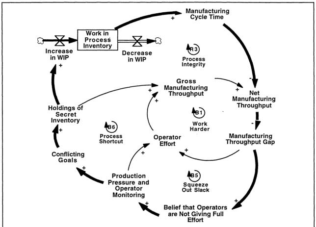
Figure 10. As throughput objectives conflict with cycle time reduction goals, workers began to hold secret caches of inventory, lengthening cycle time and reducing process capability.
