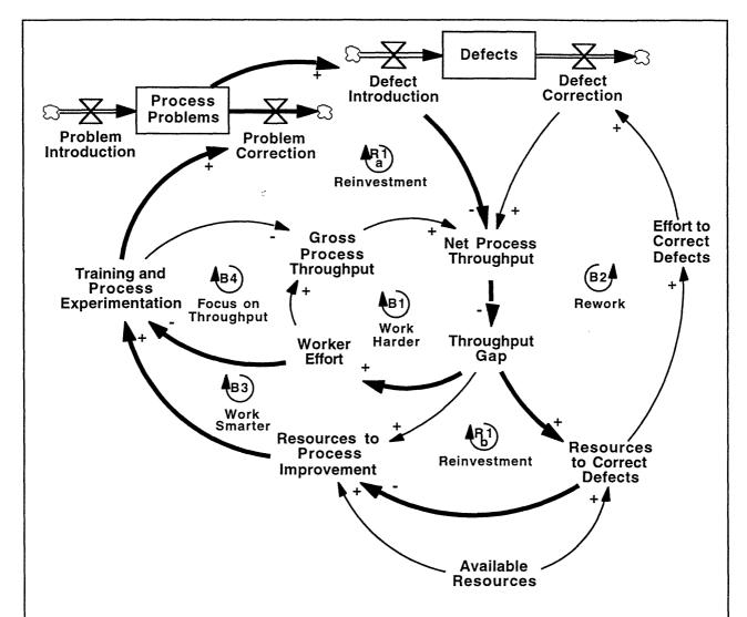
**Figure 5.** The reinforcing feedback created by finite resources: as more time is devoted to defect correction, less is available to correct process problems, leading to still more defects and still less time for improvement. Note also the balancing *Focus on Throughput* loop: workers can meet throughput goals by cutting back on improvement activity.
