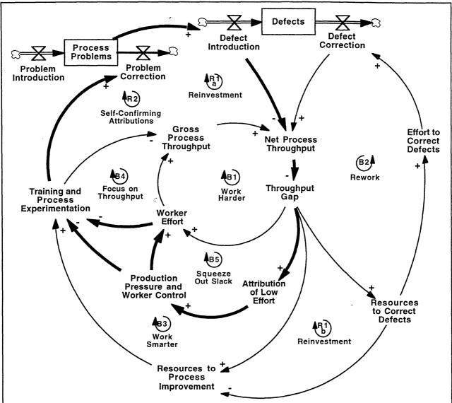
**Figure 6.** Managers who attribute the throughput gap to worker shirking will increase production pressure and monitoring in an attempt to *Squeeze out Slack* (B5). Throughput rises in the short run, but production pressure pulls resources away from improvement activity, leading to erosion of process capability and still lower throughput (reinforcing loop R2).
