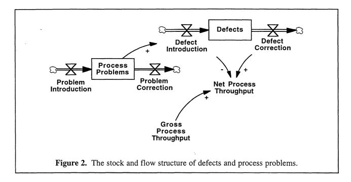
Figure two represents *Defects* and *Process Problems* as stocks (level or state variables) denoted by rectangles (Forrester 1961). A stock is the integration (accumulation) of its inflows less its outflows, denoted by the straight arrows with valves. For example, the defect stock accumulates the rate of defect introduction less the rate of defect correction:
