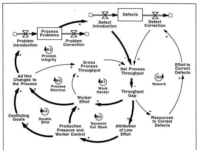
**Figure 7.** Production pressure and control over worker effort conflict, forcing workers to find work arounds, eroding process integrity and leading to still more production pressure and still tighter controls (reinforcing loops R3 and R4).
