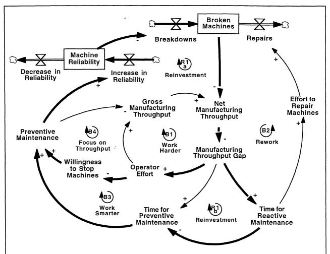
**Figure 8.** As breakdowns reduce throughput, more time is spend in reactive maintenance at the expense of preventive maintenance, leading to still more breakdowns.
