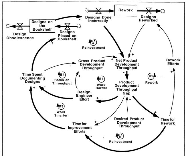
Figure 11. Development engineers under pressure to meet deadlines failed to document and share their designs. Without this learning, design error rates remained high, reinforcing schedule pressure and limiting time for future improvement.
