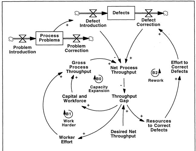
**Figure 3.** Negative feedbacks controlling throughput. The loop identifiers (e.g. B1) indicate whether a loop is a negative (balancing) feedback or a positive (self-reinforcing) feedback. See Richardson and Pugh 1981.
