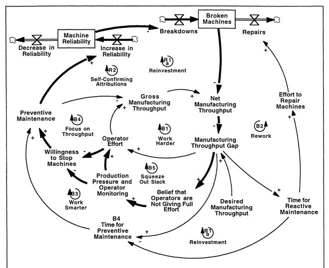
Figure 9. Boosting throughput objectives reduces the willingness of workers to stop machines for maintenance or to correct problems, leading to still more breakdowns and production pressure.
