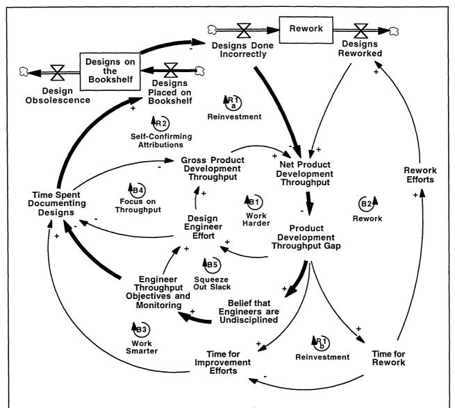
Figure 12. The belief that engineers simply needed to work harder led to aggressive throughput goals which could only be met if the engineers failed to document and share their designs, perpetuating low design productivity.
