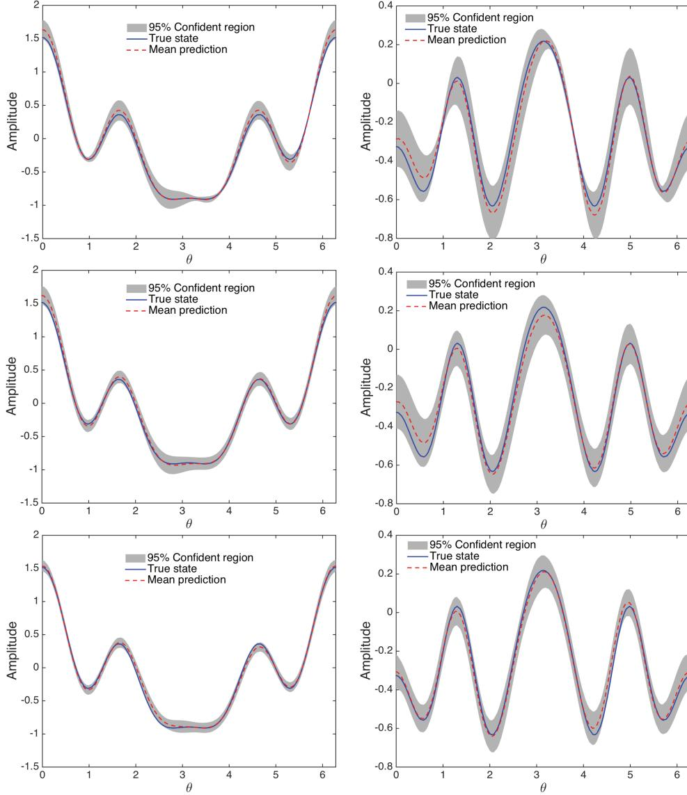
FIG. 8. Panels show the true state and the mean prediction as a function of  $\theta$ : the real part (left) and the imaginary part (right). These results are obtained using  $M = 4$  (top row),  $M = 8$  (middle row), and  $M = 12$  (bottom row) observations with  $\sigma_{\text{noise}} = 0.005$ . In these plots the shaded area represents the mean prediction plus and minus two times the standard deviation function (corresponding to the 95% confidence region).
