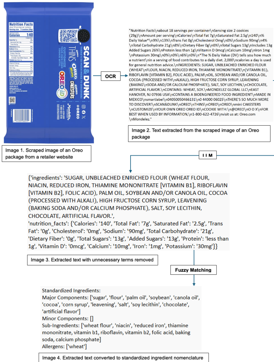
Figure 1. Diagram of the process flow of the pipeline for processing ingredient data from scraped web images.
