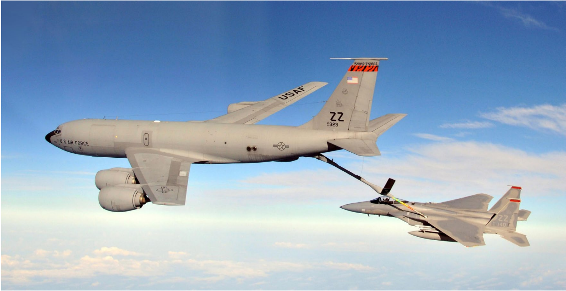
A KC-135 Stratotanker refueling an F-15
